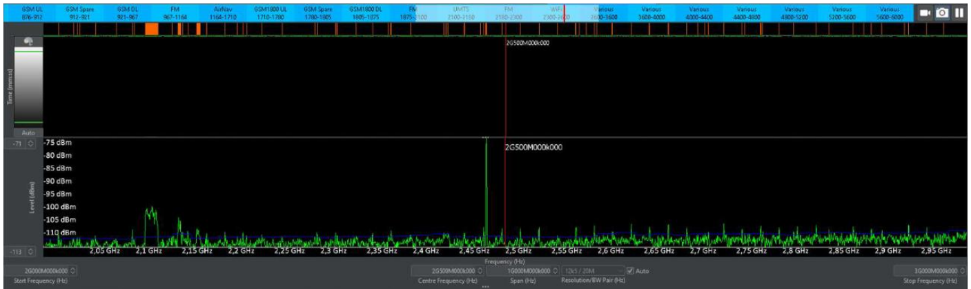
The 2-3GHz S-band shows minor interference from a nearby cellular tower.
